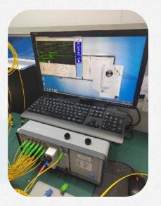
Optical Fiber Insertion Back Loss Tester
